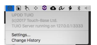
Click the "apple" logo on the top left of the menu bar and go to "About This Mac" then select "System Report" users should notice a USB device called SiS HID Touch Controller. If this device is showing in the USB but UPDD is showing No Registered Devices, then users may need to update to the latest RAVEN installer and re-install UPDD.
