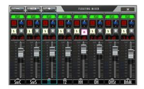
Like the RAVEN External Mixer, the floating mixer can also be banked using finger swipes. Touch the fader faceplate and glide your one finger left and/or right to bank by one track at a time. Do not touch the fader cap for a banking motion. Users can also bank more quickly by using two-fingers on the faceplate of the fader tracks and swipe left or right to bank by 24-tracks at a time. Pressing the pan button will switch the top section of the mixer from automation modes to pan modes.
