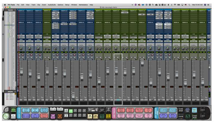
Example of Proper Alignment, notice the red line of the RAVEN is flush with the Pro Tools tracks list and the RAVEN fader colors are syncing with the color of the Pro Tools tracks and meters.
