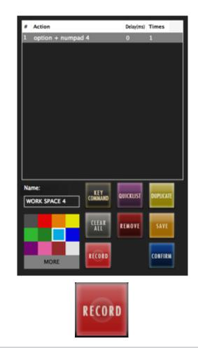
The Batch Command System Recording feature records based on the X/Y-Axis screen location.
