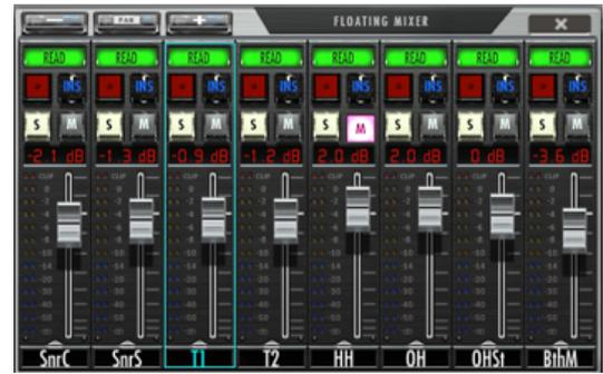
The floating mixer can be expanded or collapsed by pressing the “-” or “+” button on the floating mixer header. The mixer can be viewed as 8, 16 or 24 channels.
