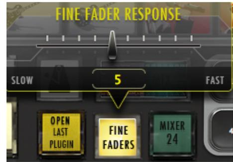
We have also included the ability to control the response of the Fine Faders by pushing and holding the Fine Faders button on the RAVEN Tool-bar. Adjust between 1 and 20, 1 being the slowest response for extreme detail and 20 being the fastest Fine Fader response time.
