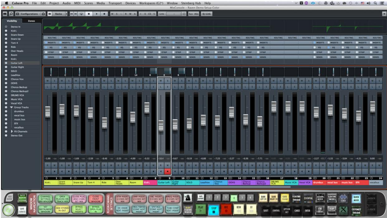
If the fader caps don't follow when widening or adding surround pans then there must be an alignment issue. Here is an example of mis-alignment, where the fader lane is to far below the red outline.
