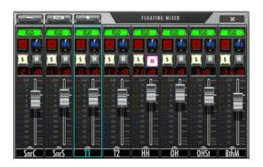
Like the RAVEN External Mixer, the floating mixer can also be banked using finger swipes. Touch the fader faceplate and glide your one finger left and/or right to bank by one track at a time. Do not touch the fader cap for a banking motion. Users can also bank more quickly by using two-fingers on the faceplate of the fader tracks and swipe left or right to bank by 24-tracks at a time. Pressing the pan button will switch the top section of the mixer from automation modes to pan modes.
