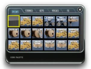
To remove an icon, touch the blank icon box in the palette, and then touch the channel icon slot you wish to remove.
